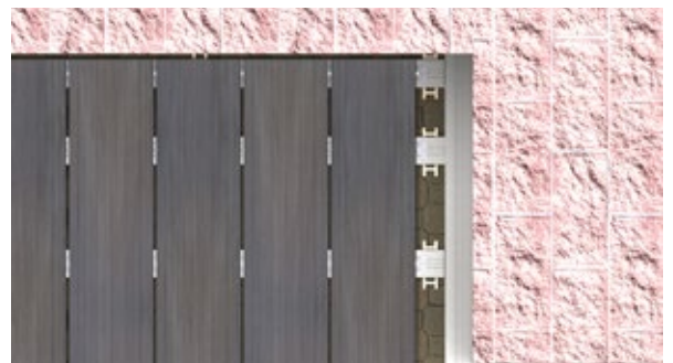
44. Gap for placing the slat. Detail.
