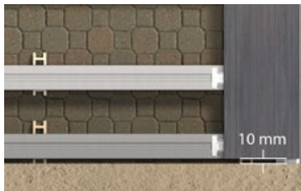
38. Separation of the headers from the deck with regard to the wall.
