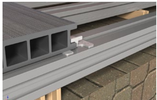
41 Clip and stainless steel screw on an aluminium batten. Deck header resting on the batten.
