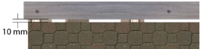
62. Minimum distance between the moulding and floor.
